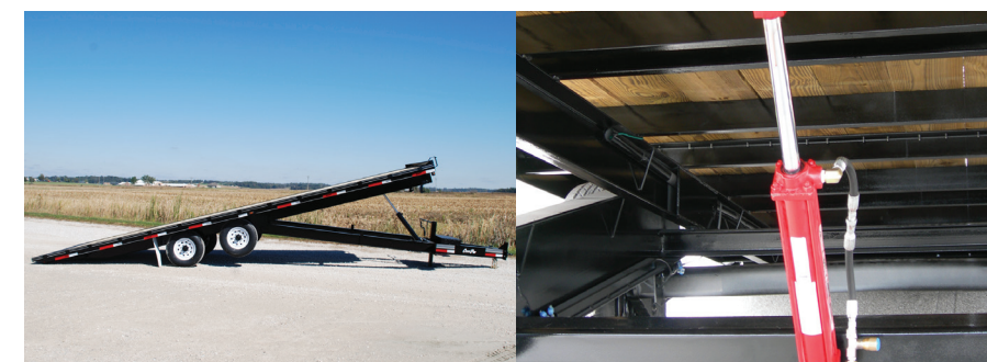
Left: Tilt trailer available as tag Right: Standard dampening cylinder on 6+21 models
